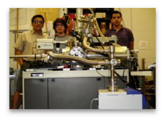
collection lens and an electron energy analyzer. Other elements include an introduction vacuum chamber, sample mounts and a data collection system. A useful additional item is an ion gun used to bombard Ar or Ne gas ions to remove surface contaminants from the sample.
