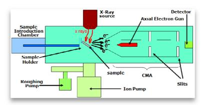
The diagram shows the main components of an XPS system such as the  $\Phi$ 560 which operates with either Al K $\alpha$  (1486.6 eV) or Mg K $\alpha$  (1253.6 eV) x rays and at a pressure smaller than  $10^{-9}$  Torr.
