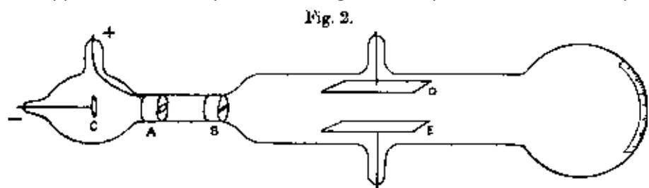
metal plug fitting tightly into the tube and connected with the earth; after passing through a second slit in another earth-connected metal plug B, they travel between two parallel aluminium plates about 5 cm. long by 2 broad and at a distance of 1.5 cm. apart; they then fall on the end of the
